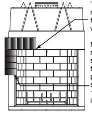
The non-combustible finishing material across the top of fireplace opening will be even with lower edge of metal face.
